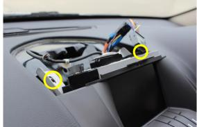
2 Remove lower storage part + unplug cable from below the stereo unit
