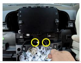
7 Install upper bracket using 2x screws removed in step 6.
