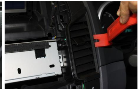
Remove centre console cover. Remove cover by pulling from the bottom out. No screws attached.
