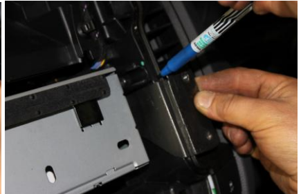
Remove centre console cover. Remove cover by pulling from the bottom out. No screws attached.
