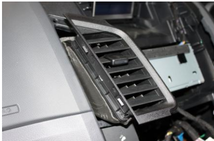
Remove centre console cover. Remove cover by pulling from the bottom out. No screws attached.
