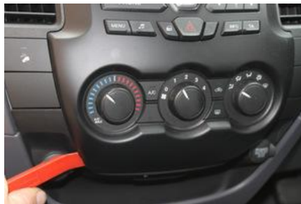
Remove centre console cover. Remove cover by pulling from the bottom out. No screws attached.
