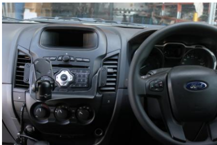
Remove centre console cover. Remove cover by pulling from the bottom out. No screws attached.
