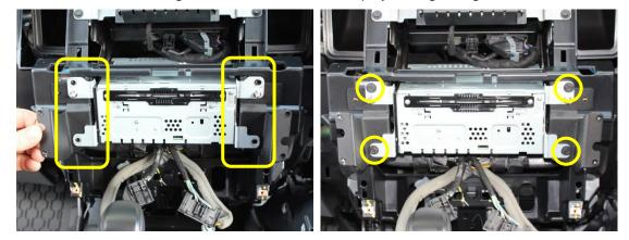
8 Measure & cut 55mm off the side tabs. Careful not to scratch or damage the front of the console
