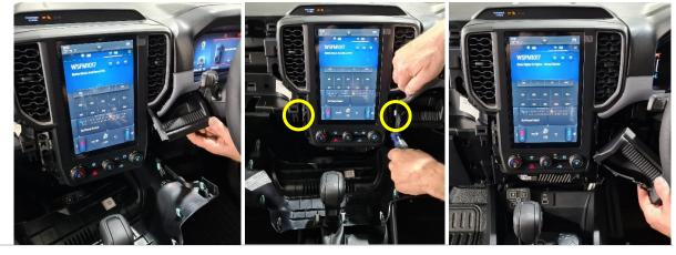
5 Using a sharp blade, carefully trim the indicated internal plastic rib as shown. Repeat for the other side.
