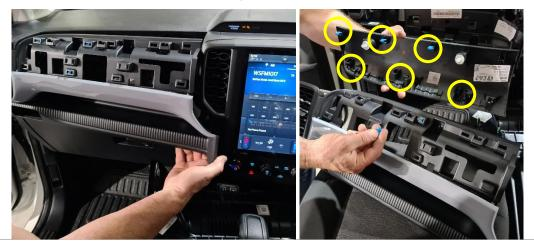
4 Loosen driver side dash piece as shown, then remove 2 x dash screws per side. Remove dash piece.
