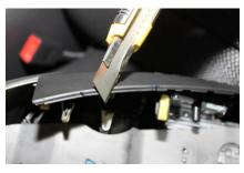
For better fit trim "internal plastic" without damaging the "exposed plastic"
