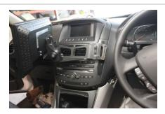
Fit Console, plug all electrical, re -screw, snap back the plastic components.
