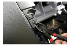
Loose screw off slightly push "U" packer under the plastic. reason is to align the plastic moulding to the centre console. Trim plastic standoff
