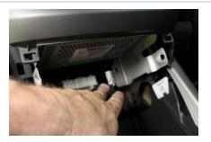
Unplug all electrical plugs. Remove screws
