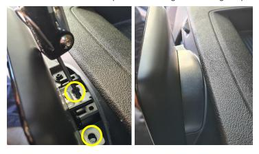
Install front dash bracket with 3 x screws provided.
