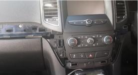
2 Remove 6 screws, 3 on each side of the control panel.
