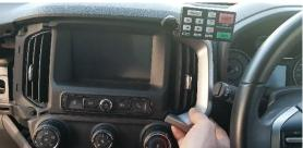
2 Remove screws, on each side of the air vents.
