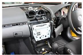
8 Install L+R side brackets onto centre console (4 screws)
