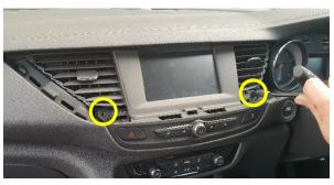
Carefully tilt centre unit forward and unplug wires.
