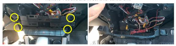
8 Install side brackets (L+R), by using existing screw at the back.
