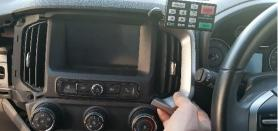
2 Remove screws, on each side of the air vents.
