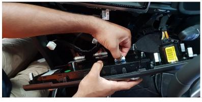
Remove 2x screws and detach plastic bar.
