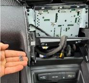
Remove 1 x screw from dash, then install second bracket as shown.
