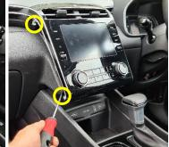
2 Loosen panel on underside of display unit. Then release unit from the dash and unplug cables.
