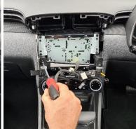
Return cables, then reinstall display unit, 4 x screws, and underside panel.
