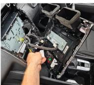
On the rear of the display unit remove 6 x screws. Install first bracket using these 6 x points.
