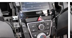
Remove 8 screws surrounding of A/C control panel
