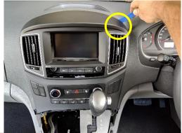
Change gear to N, ensuring handbrake is engaged. Unplug and remove A/C unit, vents and cover.
