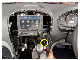
7 Change gear to N, ensuring handbrake is engaged. Plug in and replace A/C unit, vents and cover.
