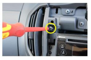
Slide in both side brackets either side of centre control unit, securing with two screws.
