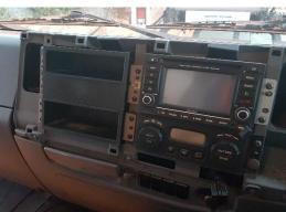
2 Unscrew and remove both lower and upper storage units
