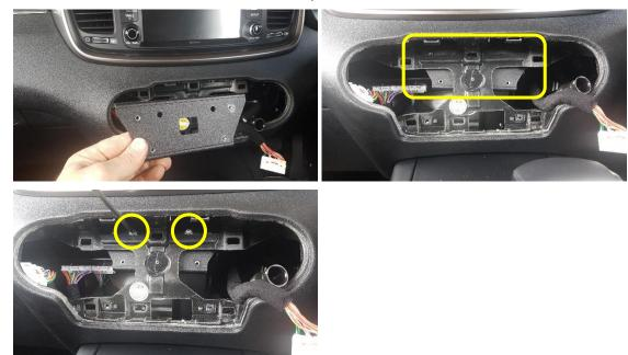
Slide flat bracket behind plastic, and secure with two screws.
