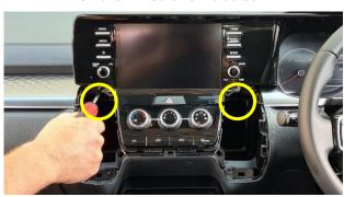
**4** Loosen screen unit, unplug cables, and set aside.
