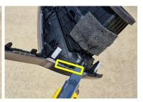
Return air vent unit to original position. Then, attach front bracket using 4 x mounting positions and screws provided.
