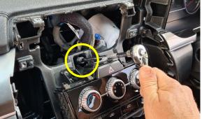
5 Place supplied bracket into place as shown and fasten into place with previously removed 1 x nut.
