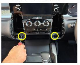
Install left and right sided brackets and fix into place using screw provided.
