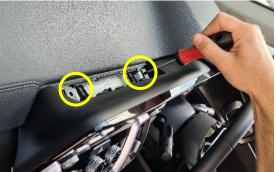
Loosen and remove air vent piece.
