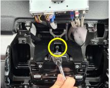
**8** Restore screen unit and previously removed screws to their original positions.
