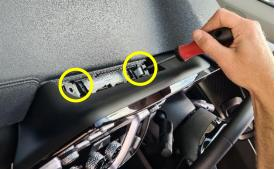
2 Loosen and remove air vent piece.
