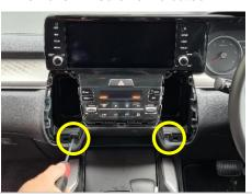
4 Place side bracket as shown. Using a sharp blade, carefully mark then trim the inner plastic like so.
