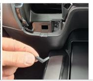
5 Install left and right-side brackets. Then, remove 2 x screws indicated.
