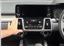
Install front dash bracket using 4 x provided screws.
