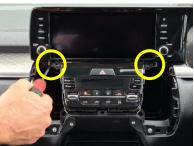
Loosen screen unit, and carefully set on the upper dash area.
