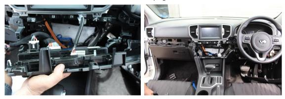
Screw in side bracket to front console
