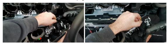
Remove 2x upper screws. Install upper bracket using these 2x existing screws.
