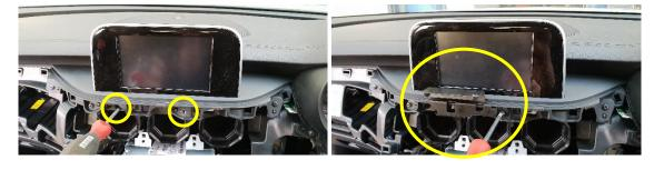
Remove 2x lower screws. Install low bracket using these 2x existing screws.
