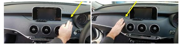
12 Centre panel tightly fitted with no gaps, If needed, can trim plastic rib on the inside lower.
