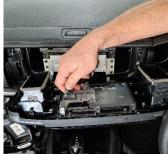
2 Remove 2 x dash screws, then install first bracket in place.
