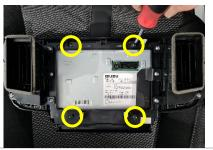
5 Plug in and reinstall control unit and air vents.
