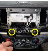
Remove 5 x screws and detach screen. Move second bracket into place.
