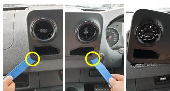
4 Place and secure upper bracket at 2 points using self tapping screws provided.
