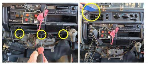
Install first bracket using 2 x existing internal screw locations.
