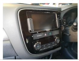
7 Install dash bracket with 4x countersunk M5 screws provided.
