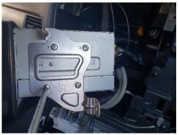
4 Install Left & Right side brackets, using the existing 8 screws (4 screws each side).
