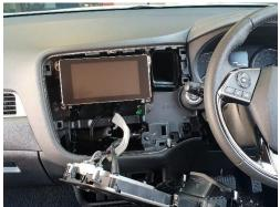
2 Remove 4 x screws and lift out centre control unit.
