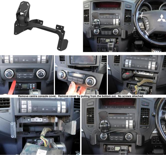
Install the side tabs as shown, Screw 4 x self tappers screws into the side and replace the console cover snap fit. Place the front dash bracket with screws provided.
