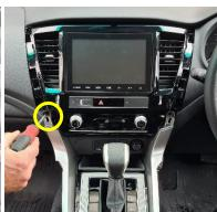
Loosen central dash unit, remove cables and set aside.
