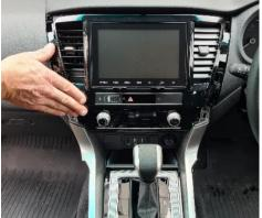
Install lower bracket using previously removed 1 x screw. Using a sharp blade carefully shave away inner plastic from the indicated area to allow a snug fit for the bracket.
