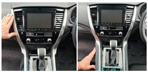
Install front bracket using 3 x countersunk screws provided.
