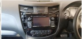
Carefully tilt lower control unit forward.
