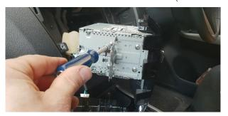
7 To install side bracket, slide existing bracket underneath, securing with existing screws.
