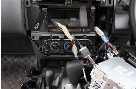
5 Unscrew 4 screws from the head-unit mounting brackets. Place the In-Dash Mount side brackets between the siver mounting brackets and the head unit then reinsert the screws.
