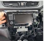
3 Remove screws from 3 x locations, then install side bracket. Place display unit back into dash.
