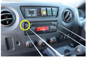
2 Loosen the stereo unit forward
