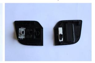
10 Cut plastic lip on either side of centre console. Be careful not to damage the front fascia.
