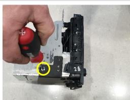
Install L + R side brackets using remaining 2x screws from each side.
