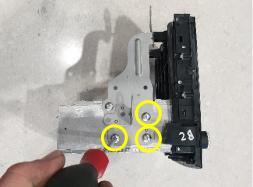
Install lower bracket using 1x screw from each side, as pictured.
