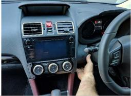
14 Install front bracket using 4x black screws provided.
