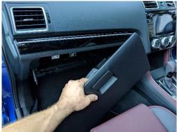
2 Remove screw from inside compartment on right side, as pictured.
