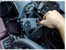
Replace centre console and A/C vents, replacing screws removed in Step 7.
