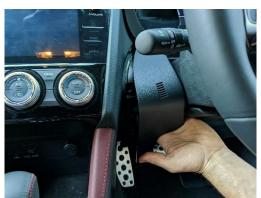
Start engine to rotate steering wheel, remove one screw on each side.
