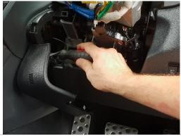
7 Carefully pry and remove upper A/C air vents, without unplugging, and remove 2x screws.
