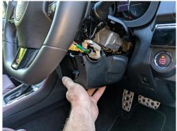
Replace 2x screws removed in Step 4 beside steering wheel, and replace screw removed and panel loosened in Step 3.
