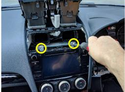
8 Remove centre console, without unplugging, and remove 4x existing screws on each side.
