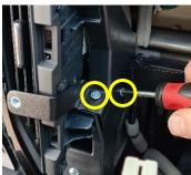
Return display unit and 4 x screws to the dash.
