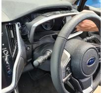
2 Remove passenger side dash piece and driver side dash piece as shown. Then, loosen upper dash piece and set aside.
