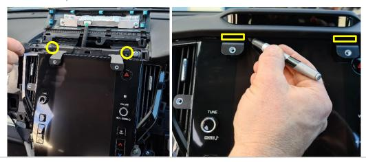
**7** Remove the upper dash piece from the dash. Using a sharp blade, carefully trim 2 x locations.
