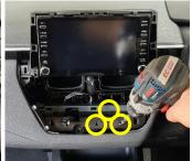
5 Install small bracket in behind, fixing into place using 3 x supplied screws. Then, replace 1 x screw.
