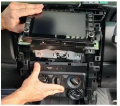
Set display unit back into dash. Replace 4 x screws and plastic cover piece.
