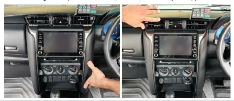
Install front bracket using 4 x mounting locations.
