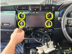
6 Loosen display unit and carefully set it down. Remove 2 x indicated screws from each side.
