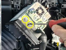
8 Separate upper cover from the AC controls as shown. Then, place AC controls into the dash.
