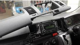
2 Remove 4 x screws and lift out centre control unit.
