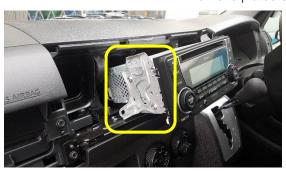
4 Install side brackets using 8 screws (4 screws each side).
