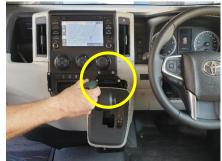
10 Attach upper part of right bracket to lower part, Install front bracket using 4x black screws provided.
