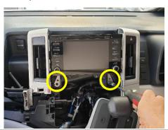
4 Install left bracket using existing screw removed in step 4, and 2x silver screws provided.
