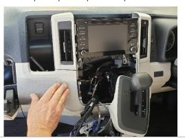
Install lower part of right bracket using 1x screw removed in Step 4. 7
