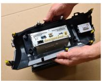
Remove sticker on inside edge of plastic as shown.Using a sharp blade carefully trim away 3 x ribs. Repeat both steps for the other side.
