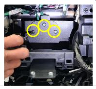
**9** Replace all previously removed plugs and reinstall display unit into the dash.
