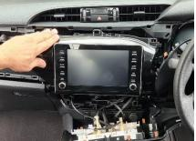
10 Replace 4 x screws around display, then place AC unit back to original position.
