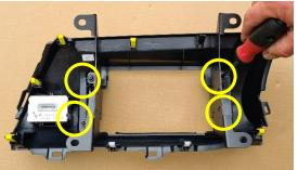
9 Place plastic cover back around display unit. Then, replace 6 x side screws.
