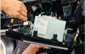
Remove 4 x screws on rear of display unit.
