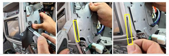
4 Install bracket in place. Repeat process and install opposite side bracket. Reinstate dash pieces.
