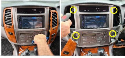
Loosen central unit and remove 4 x screws.
