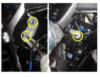
4 Remove air vents and screws on either side. 6 x In-total screws. 4 x In front & 2 x Inside
