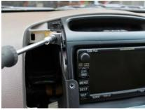
Trim one piece of plastic sticking out on both sides. See photo. Remove 4 bolts
