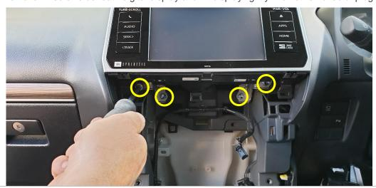
Slide L+R brackets under the digital display metal tabs, as pictured.
