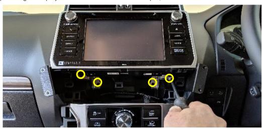
Replace screws on L+R sides removed in Step 3.
