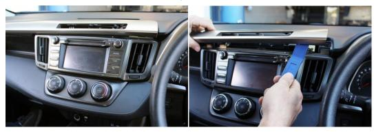
2 Remove vent from both sides of the head unit
