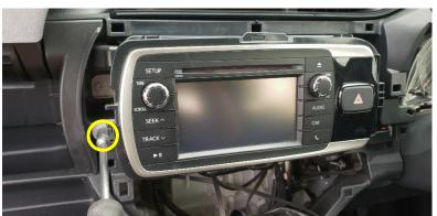
**5** Lever and lift plastic from hazard light control.
