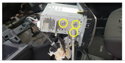
Install side bracket using 3x screws, removed in Step 11.
