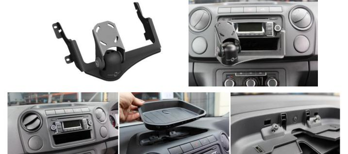
Pop top cover, 2 x remove screws, Pop 2 x disc on the side as shown on photo, remove cover.
