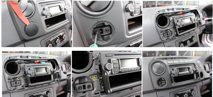
Attached the two side brackets, snap back the front plastic cover and components. attached the front Indash mount :-)
