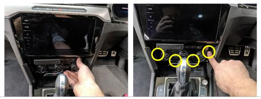
**14** File down plastic tabs on the plastic trim around A/C controls, as shown. Remove plastic up to metal tab on the back side. Do not remove any metal.
